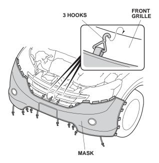
3. On each side, insert six tabs between the headlight and the grille.
